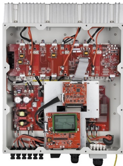
▲ Small, low in weight, compact and highly efficient: The 20000TL3-HE, a 20 kW inverter made by Growatt, achieves high maximum efficiencies despite its rather Spartan equipment features. The thermographic image shows component temperatures of up to 80 °C on the circuit boards (on the surface of the grid disconnect relay). The two electrolytic capacitors that are visible are, in contrast, in the green or, in this case, the blue part of the temperature scale.
